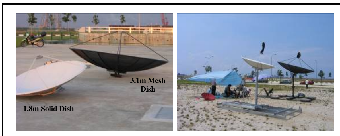
Figure 6 : FSS satellite dish set up at the field test.
